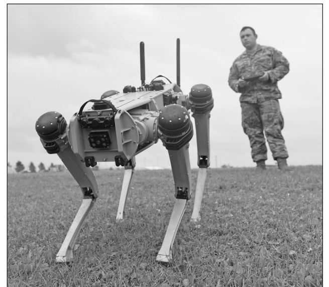
Master Sgt. Krystoffer Miller, 325th Security Forces Squadron operations support superintendent, operates a Quad-legged Unmanned Ground Vehicle at Tyndall Air Force Base, Fla., March 24, 2021. The purpose of the Q-UGV is to add an extra level of protection to base.U.S.
