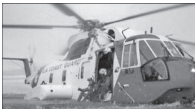
Sikorsky HH-3F Pelican entered service in 1967. Its twin turbine (max speed 142 knots) medium range (650 NM) amphibious specifications extended CG offshore search and rescue capabilities. This helicopter type was transferred from Salem to Cape Cod in 1970.
